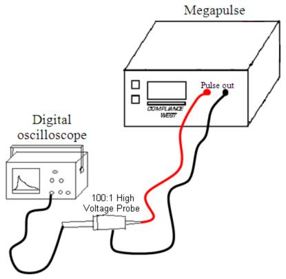
Figure 3. Waveform Measurement Setup
